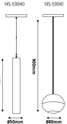
Volt: **48V DC 50/60Hz** • LED Type: **COB SMD1313**
